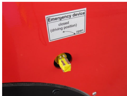
Emergency device „opened“ (vehicle can be lowered)
